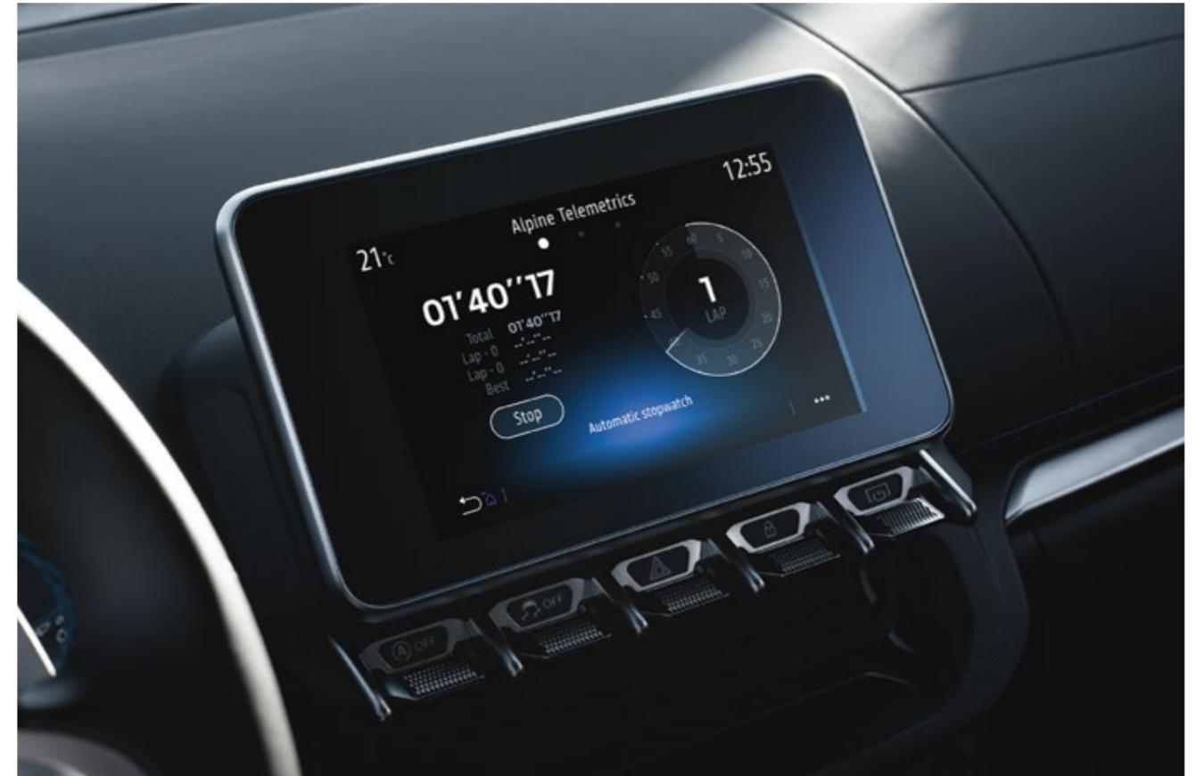
Alpine Telemetrics provides real-time access to technical data recorded by the vehicle's sensors (pressures, temperatures, engine speed, steering wheel angle, etc.) and presents it via digital graphs. In addition, the integrated chronograph allows you to measure lap timing and performance.
