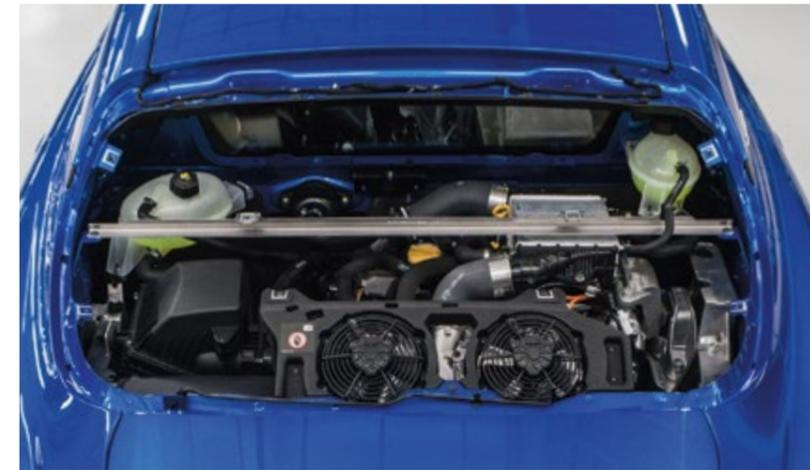
Tuned by Alpine powertrain engineers, the 1.8-litre direct injection engine delivers thrills and strong performance. The new 300 hp engine offers a torque of 340 Nm generously available from 2,400 to 6,000 rpm, accelerating (A110 R version) from 0 to 100 km/h in 3.9 seconds and reaching up to 285 km/h on track.
