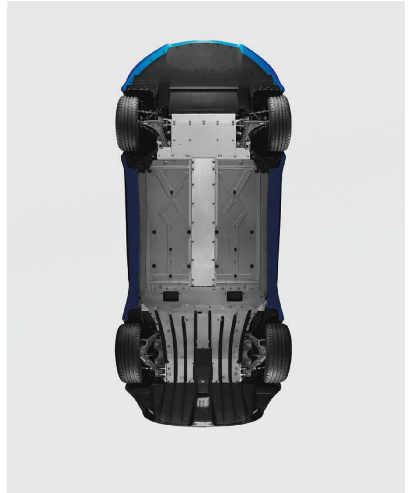
Alpine engineers have also paid particular attention to the aerodynamic development of the Alpine A110, using technical solutions borrowed from the world of racing. Thus, the A110 features an integral flat floor, a technique carried over from the world of high-level motor racing. Thanks to a rear diffuser located beneath the rear bumper, the A110 offers excellent rear handling.
