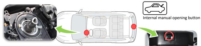
Steering column : Hollow and breakable with tools
