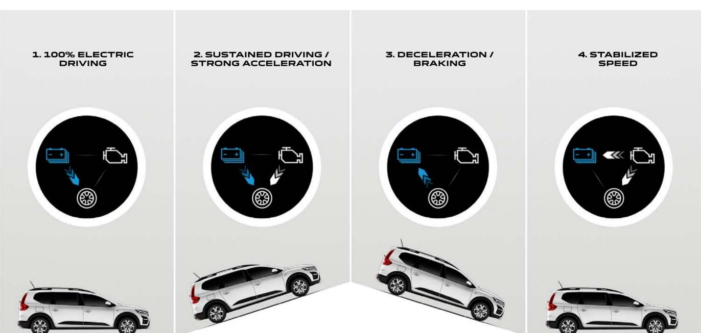
1. 100% electric driving: only the electric motor drives the wheels.
