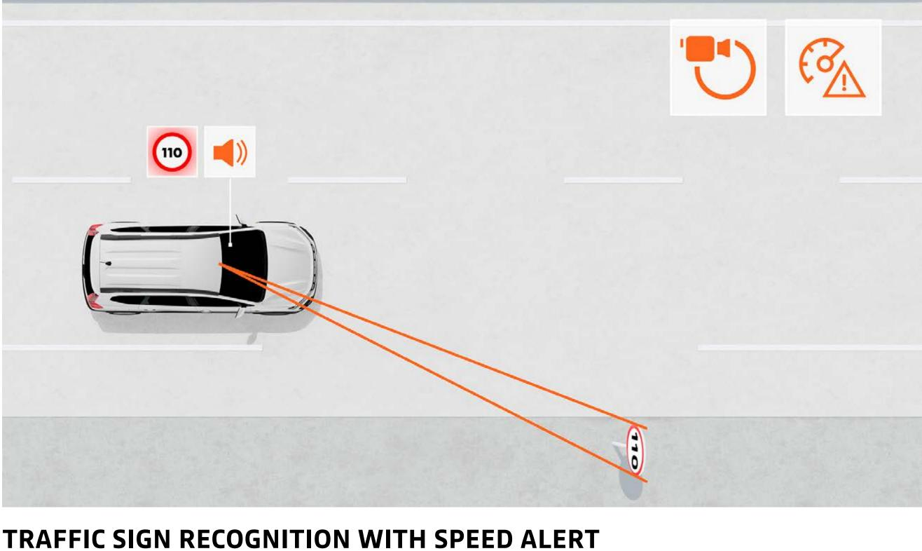
This system provides a reliable real-time indication of the maximum speed on the road and warns the driver if they exceed the speed limit with visual and audible alerts (which can be disabled).
