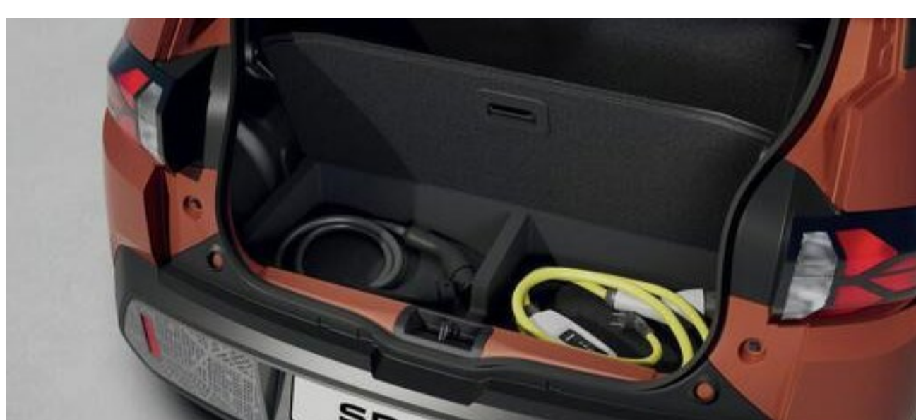
Double floor for cable storage
