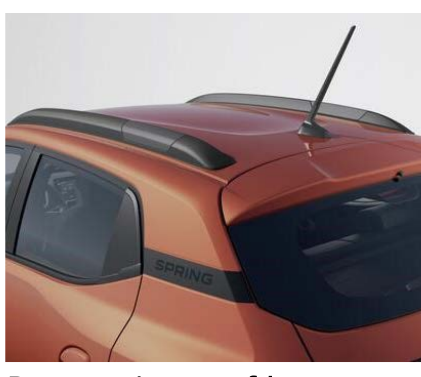
Decorative roof bars (Not load bearing)
