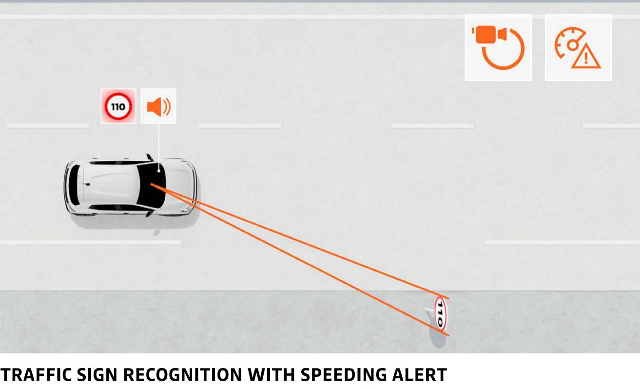
This system provides a real-time indication of the maximum speed on the road and warns the driver if they exceed the speed limit with visual and audible alerts (which can be disabled).
