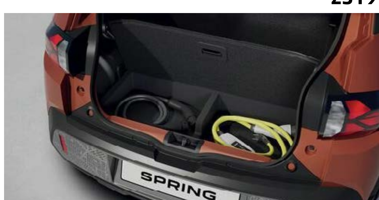
Double floor for cable storage
