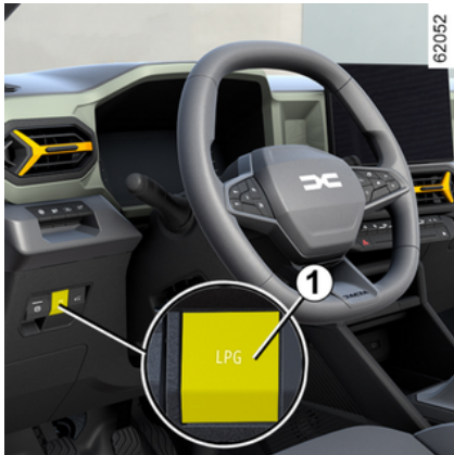
LPG/petrol fuel mode selection control 1
