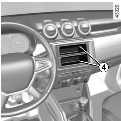
Centre console storage compartment 4 (or radio location)
