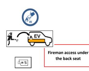
If traction battery on fire → Water extinguishing by filling
