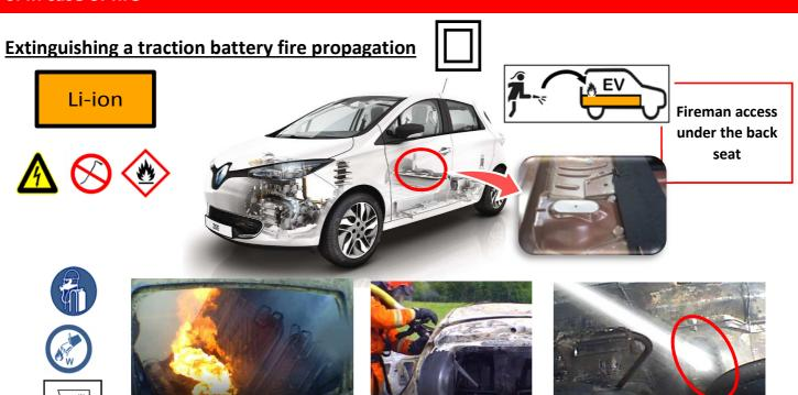
If traction battery on fire : → Water extinguishing by filling
