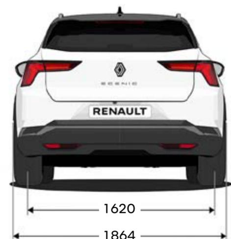
Abmessungen in mm
