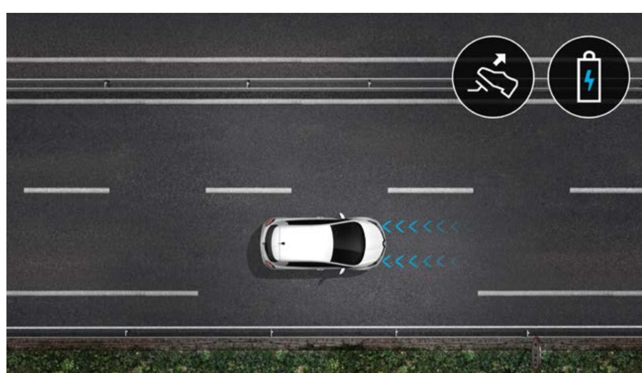
regenerative braking Regenerative braking allows the battery to charge by recovering energy as soon as you take your foot off the accelerator. In mode B, this braking is more intense and allows you to drive in a more economical way that requires less use of the brake pedal.
