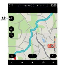
When a route is in progress, use the **38** control to return to the cursor position after moving around the navigation map.
