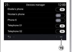
Using the "Devices manager" 17 function, you can select the telephone which you wish automatically to connect to "smartphone replication".
