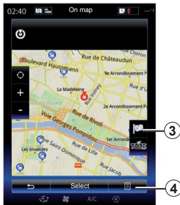
Move around the map to position the cursor on your destination, then confirm by pressing “Select”: the system calculates the route.
