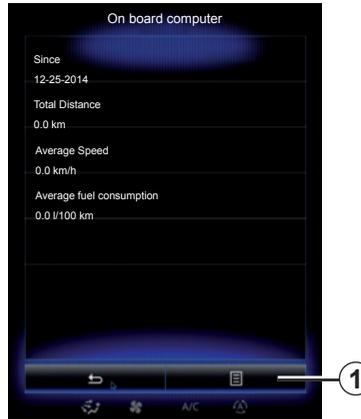
To reset the on-board computer and instrument panel information, press **1** then “Reset”.
