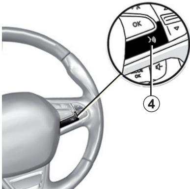
Once the “Android Auto™” application or the “CarPlay™” service is activated on your multimedia system, you can use the voice recognition button in your vehicle to control some functions of your smartphone by voice. To do this, press and hold button **4** on the steering wheel of your vehicle (for more information, refer to the section on “Using voice recognition”).
