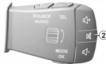
You can interrupt the voice synthesizer when using voice recognition by pressing the **2** button on the steering column control. A beep indicates that you may speak.
