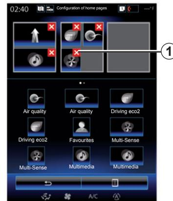
Press and hold the desired widget, drag and drop it onto one of the three home pages to be displayed.
