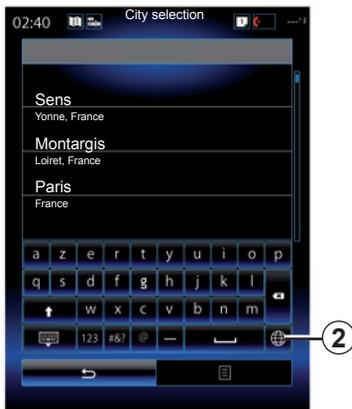
You can change the type of keypad on the multimedia system by pressing the 2 button (“ABC”, “Qwerty”, “Qwertz”, etc.).
