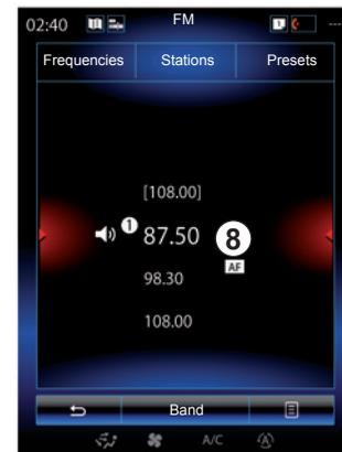
The names of the radio stations that do not use the RDS system or if the vehicle is located in a bad radio reception area, they will not appear on the screen. Only their frequency is displayed and sorted at the beginning of the list.
