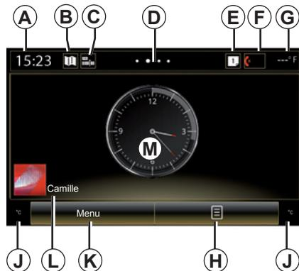
**E** “Suggestion bar” and “Notifications” shortcuts: direct access to information on your vehicle’s connectivity, to Bluetooth® devices connected to the multimedia system and the notifications of the connected telephone.
