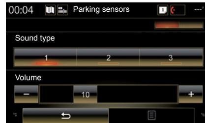
**Note:** if the "Sound alert" function is set to "OFF", the "Sound type" and "Volume" functions are disabled.
