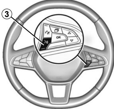
Once the "Android Auto™" application or the "CarPlay™" service is activated, you can use the voice recognition button in your vehicle to activate some of your smartphone functions by voice. To do this, press button 3 on the steering wheel of your vehicle (for more information, refer to the section on "Using voice recognition").
