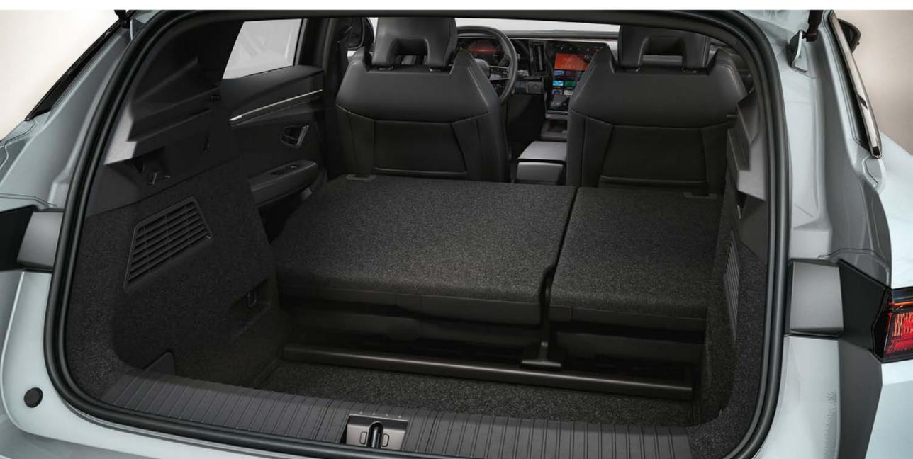
the rear seats can be folded down in 1/3-2/3 split configuration, while the passenger seat can be reclined to 45°.
