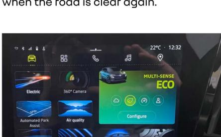
**eco mode.** This function makes the car as environmentally efficient as possible. It acts upon certain power consuming systems in the vehicle (heating, air conditioning, power-assisted steering etc.) and on power-driven actions (acceleration & gear changing).
