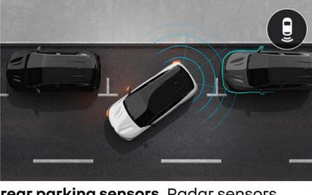
**rear parking sensors.** Radar sensors facilitate your manoeuvres by warning you with audio and visual signals about nearby obstacles to the rear.
