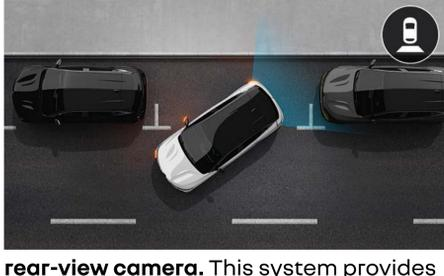
**rear-view camera.** This system provides a rear view on the screen when you engage the reverse gear. Superimposed outlines make your manoeuvres easier and safer.
