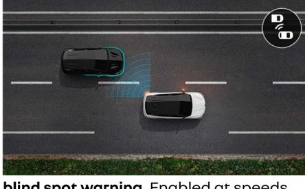
**blind spot warning.** Enabled at speeds over 15kph, this system uses warning lights to alert you about the presence of vehicles that are not visible in your field of vision.
