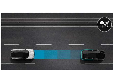
**adaptive cruise control.** This system keeps a safe following distance with the vehicle in front. It activates the brakes when you get too close, and accelerates when the road is clear again.
