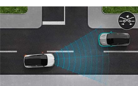
**automatic emergency braking.** This system detects vehicles to the side or in front, then stops the vehicle in the event of any danger.
