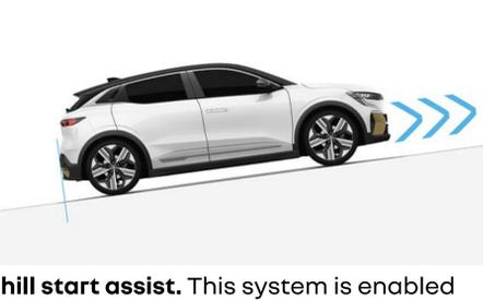
**hill start assist.** This system is enabled when the gradient is steeper than 3% by maintaining the brake pressure for two seconds.
