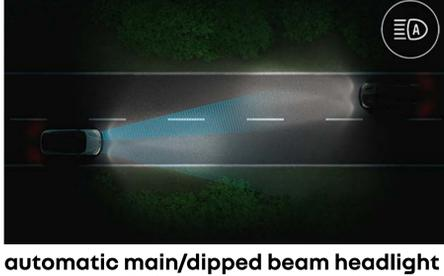
**automatic main/dipped beam headlight activation.** This system uses a camera that analyses light flows based on lighting and traffic conditions.
