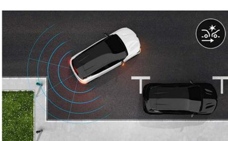
**automatic emergency braking when reversing.** This system detects obstacles at the rear and stops the vehicle automatically in the event of danger.
