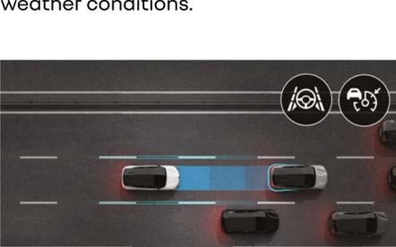
**active driver assist.** It regulates the speed by taking into account what's on the road, maintains safe distances and ensures lane centering. During slow traffic the vehicle stops and starts automatically.
