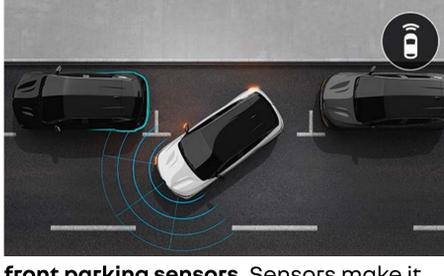
**front parking sensors.** Sensors make it easier to manoeuvre by providing you with audible and visual signals about nearby obstacles in front of the vehicle.
