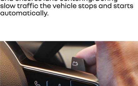
**paddle shift levers for regenerative braking.** Shift the lever for regenerative braking, this allows the driver to choose between different regenerative braking modes to suit the driving conditions.
