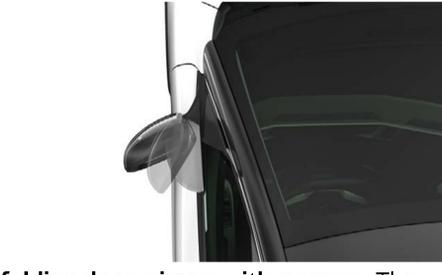
**folding door mirrors with memory.** They fold down automatically, memorising your profile and the tilt function when reversing.
