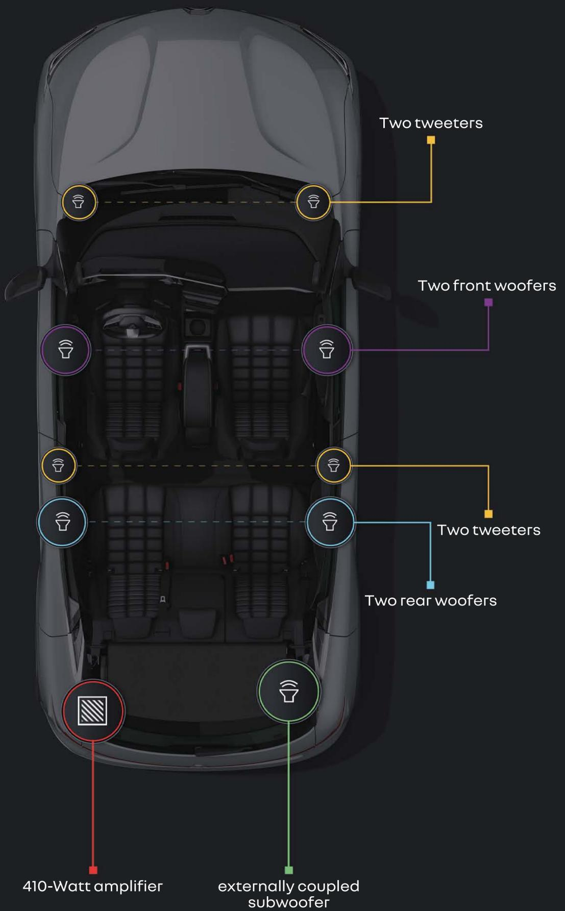
The new Harman Kardon\* sound system delivers sound via two tweeters on the sides of the dashboard, two woofers in the front door panels, two tweeters and two woofers in the rear door panels and a subwoofer in the boot. Thanks to Quantum Logic Surround™ technology and five available sound environments, any music becomes an unforgettable treat.
