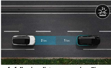
**safe following distance warning.** The front radar calculates safety distances and triggers an audible and visual warning in the event of a risk of collision.
