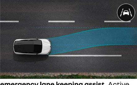
**emergency lane keeping assist.** Active from 65kph, this system uses the front camera and the front radar to detect: a risk of frontal collision with an oncoming vehicle when the driver starts to overtake or a risk of leaving the road, even where there are no roadside markings.
