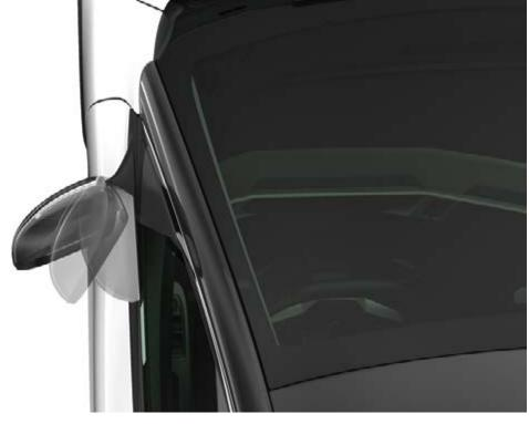
folding door mirrors with memory. They fold down automatically, memorising your profile and the tilt function when reversing.
