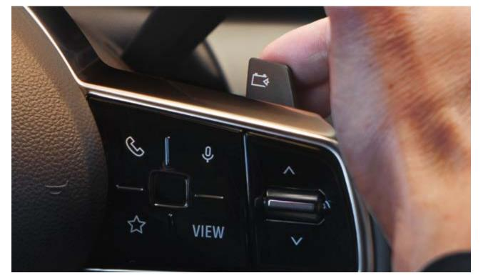
paddle shift levers for regenerative braking. For the convenience of the driver, this allows the driver to choose between different regenerative braking modes to suit the driving conditions.
