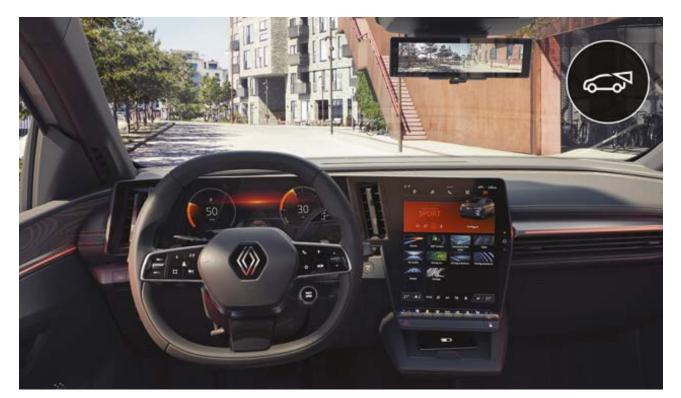
**smart rear-view mirror.** This system gives you a complete view of the rear on your central rear-view mirror.
