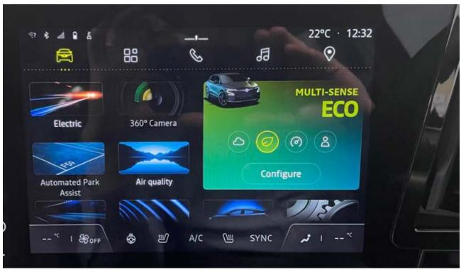
**eco mode.** This function makes the car as environmentally efficient as possible. It acts upon certain power consuming systems in the vehicle (heating, air conditioning, power-assisted steering etc.) and on certain driving actions (acceleration & gear changing).
