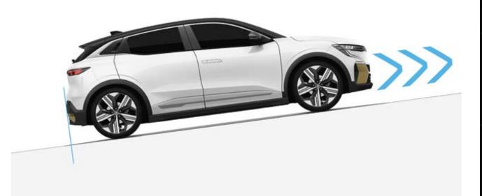
hill start assist. This system is enabled when the gradient is steeper than 3% by maintaining the brake pressure for two seconds.
