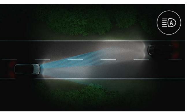
automatic main/dipped beam headlight activation. This system works using a camera that analyses light flows based on lighting and traffic conditions.
