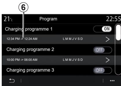
Set the charging start and end times as well as the days to which these times will apply. Press “Close” to confirm.
