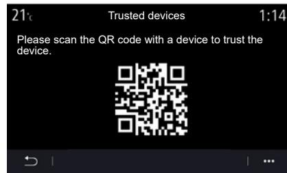
You can approve a new device by scanning the system QR Code using your telephone.
