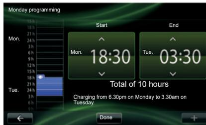
To modify the charging programmer (by week), press the “Change” button located underneath the “Calendar”. Press “Add a charge schedule” and a window will open to adjust the charge start time and end time.
