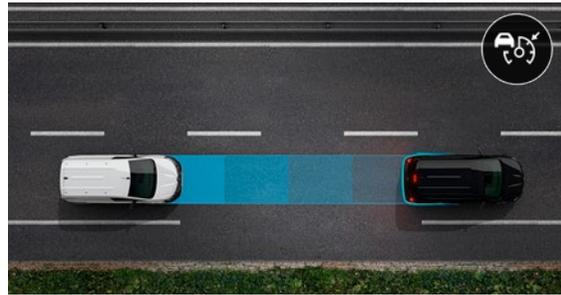
**adaptive cruise control.** This system helps you maintain a safe distance between you and the vehicle in front of you while driving. The system operates the brakes when the distance is too short and the accelerator when the road is clear again.
