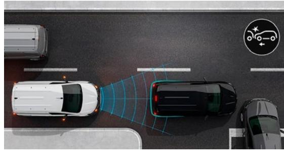
**active emergency braking system with vehicle detection.** This system detects vehicles to the side or in front, and stops the vehicle in the event of any danger. Driving in the city has never been so safe, day or night.
