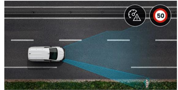
**road sign recognition and speeding alert.** This system informs you of speed limits via the instrument panel and alerts you if you exceed the speed limit thanks to a camera positioned at the top of the windscreen.
