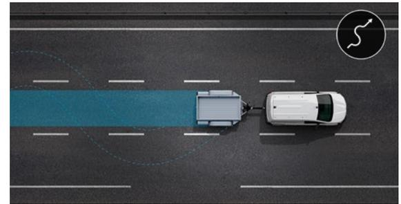
**trailer sway assist.** Trailer sway assist helps you control your trajectory when towing a trailer. The system reduces its weaving without reducing speed, and improves road holding in difficult cross-winds or poor road conditions.
