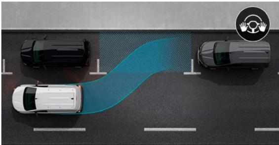
**park assist systems.** Driving has never been so easy. The front, rear and side parking sensors warn you with audible and visual signals when obstacles are close by. Hands-free parking performs all the manoeuvres for you. All you need to do is manage the speed.
