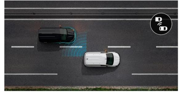
**blind spot warning.** Active above 15 km/h, this system uses warning lights to alert you to the presence of vehicles that are not visible in your field of vision.
