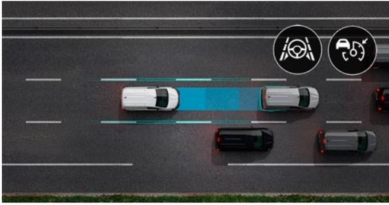
**highway and traffic jam assist.** Adjust your vehicle's speed and trajectory to the surrounding traffic. Active between 0 - 160km/h, this system regulates your speed, maintains a safe distance between you and the vehicle in front and helps you stay in your lane. When traffic slows down, the vehicle automatically stops and restarts for greater comfort and peace of mind.
