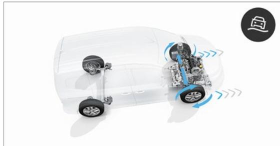
**Grip Xtend.** It allows you to drive in all weathers on different types of terrain (mud, leaves, rough roads, etc.). The system combines electronic stability control (ESC) and all-weather tyres to bring you enhanced traction, available at speeds of up to 50km/h.
