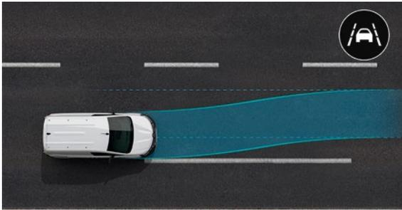
**lane keeping assist.** Active between 65 and 160 km/h, this system corrects the steering wheel to return the vehicle to its lane if you ever cross a continuous or broken line without activating your indicator.
