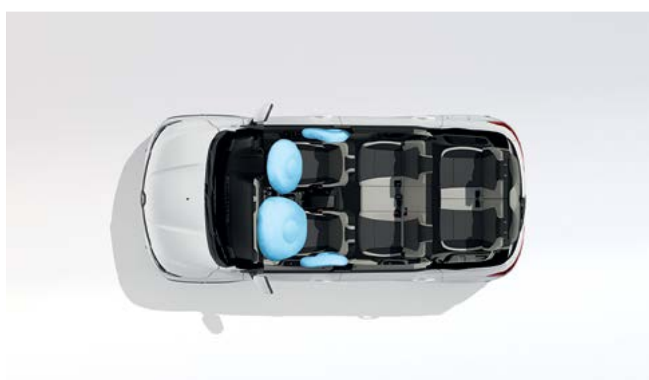
front & side airbag 1 - driver & passenger Four airbags offer increased protection.
