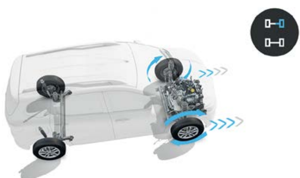
traction control system Limits wheel slip during starting, acceleration and braking.
