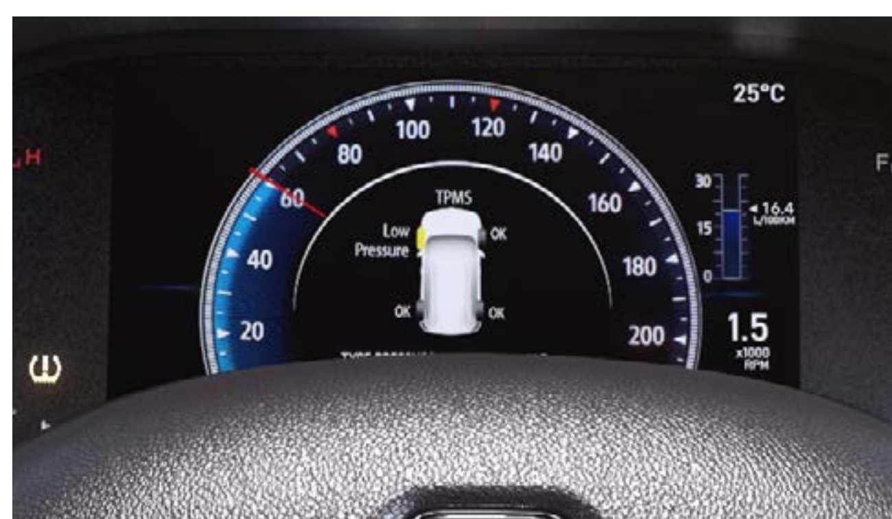
tyre pressure monitoring system Displays the tyre pressure status in real-time.
