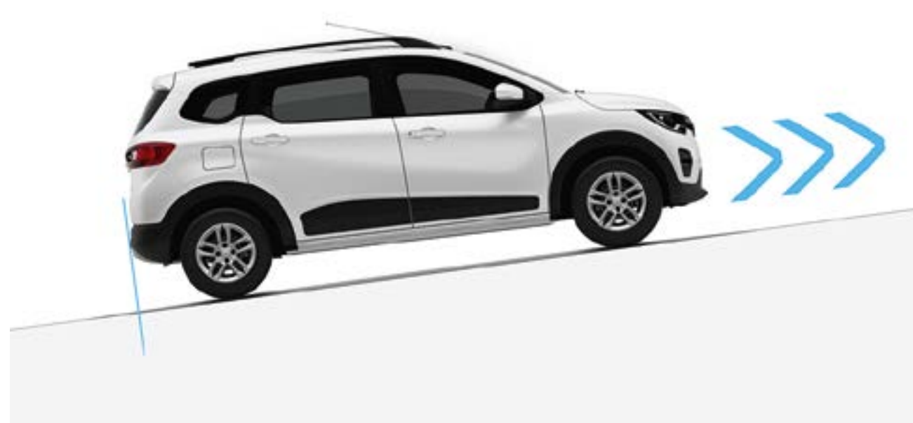
hill start assist Maintains brake pressure for two seconds, preventing rollback when you move away on a steep slope.
