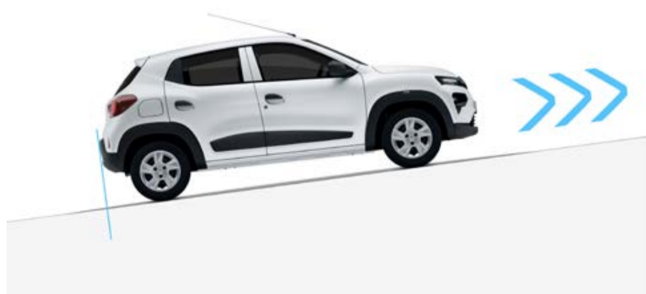
hill start assist 2 Maintains brake pressure for two seconds, preventing rollback when you move away on a steep slope.
