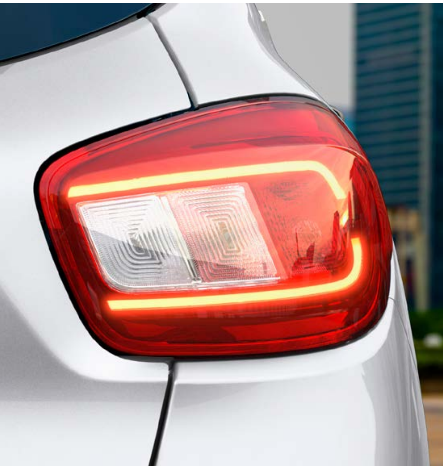
tail lamps with LED light guides
