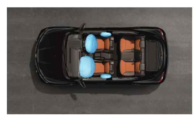
front & side airbag - driver & passenger<sup>1</sup> Four airbags<sup>1</sup> offer increased protection.
