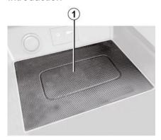
The induction charging area **1** can be used to charge a telephone without a cable.
