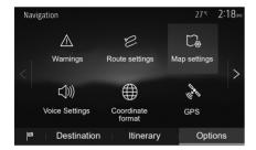
The "Options" tab at the bottom of the "Navigation" menu enables you to change the map display or the navigation settings.
