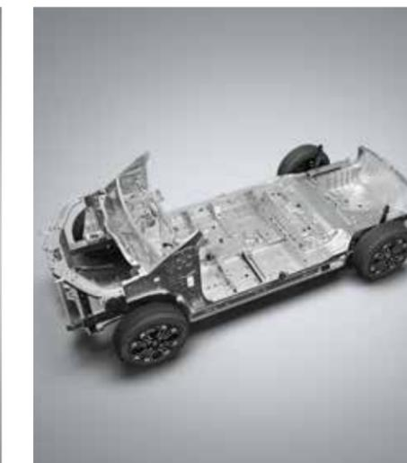
high tensile steel body with anti-roll bar
