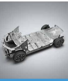
high tensile steel body with anti-roll bar
