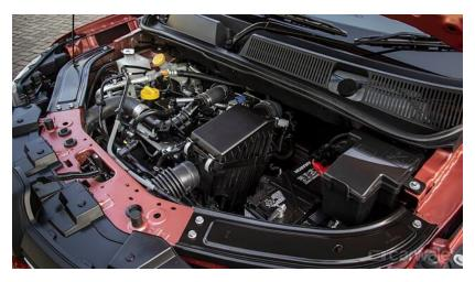
The updated Kiger continues to be offered with two engine options. The 1.0-litre non-turbo version makes 71bhp and 96Nm. It's either available with a five-speed manual or an AMT. What we are driving is the 1.0-litre turbocharged engine which has an output of 99bhp. It's available with a manual which has 160Nm, while the automatic is a CVT with a torque figure of 152Nm.
