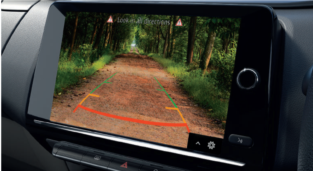
reverse parking camera with guidelines
